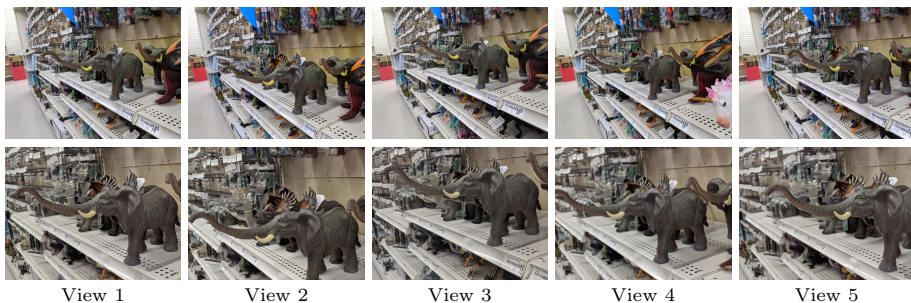
Fig. 9: Example capture from our data collection rig. Top: Views from the main cameras of the five phones on the rig. Bottom: Views from the telephoto cameras. All ten views are used to compute ground truth depth using multi-view stereo techniques.
