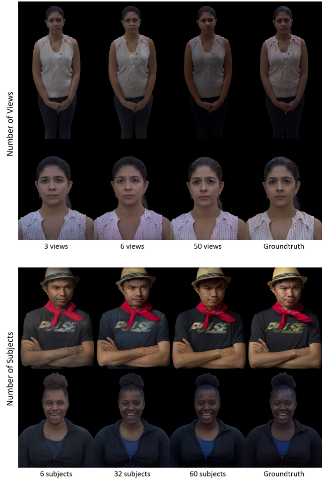
Fig. 18. Relighting results for models trained with a different number of viewpoints (top) and subjects (bottom). Increasing the number of camera viewpoints slightly improves the overall quality, especially for full body portraits. A large and diverse training dataset with many photographed individuals improves model generalization and relighting results.
